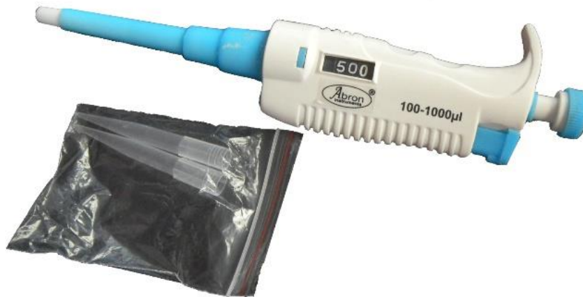
Figure 5.10. A pipette is used to very accurately displace a volume of liquid
