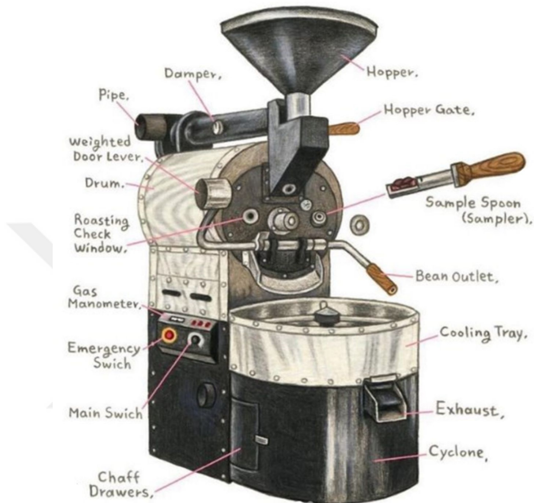
Figure 2.6. Components of a Shop-Type Coffee Roaster
