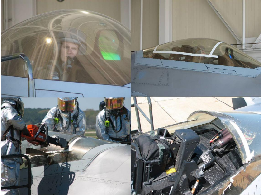
Figure 1.6 F-22 canopy failures [12]
