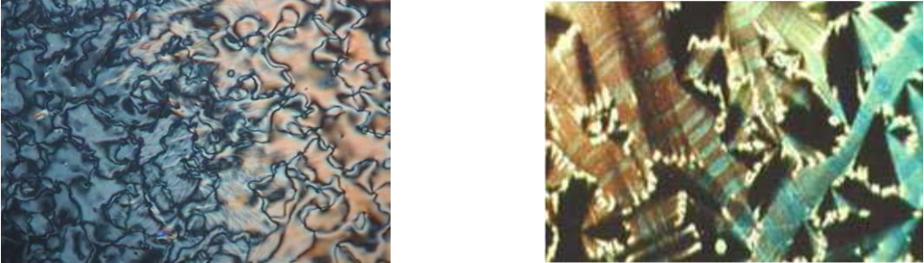
Figure 2.13 : Broken fan-shaped structures of SmC phase.
