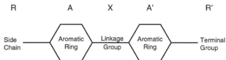
Figure 2.5 : General representation of the structure of liquid crystal molecules.
