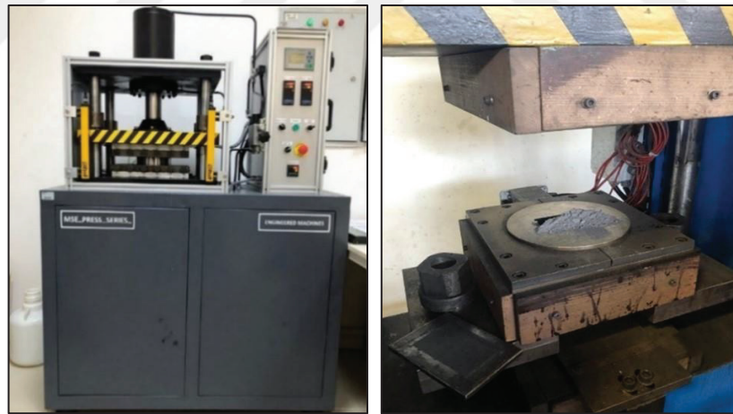
Figure 3.4. Pressing Process in Hydraulic Press Machine
