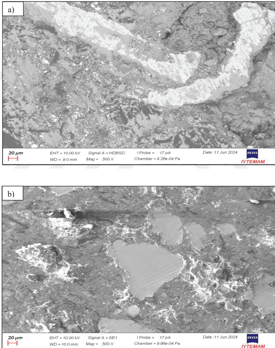
Figure 4.20. SEM Images of Sample1, a) From the Worn Surface, b) From the Sectioned Surface
