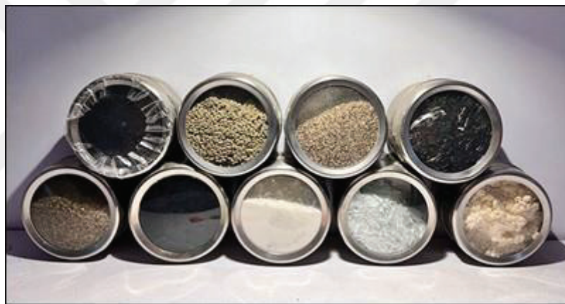
Figure 2.4. Materials Used in Composite Clutch Facing (Source: Hee et al. 2005)
