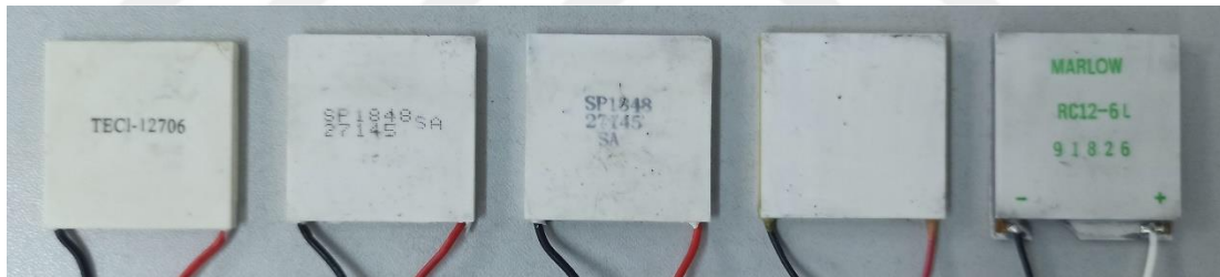
Figure 4.1. Ceramic plated TEGs from left to right labeled TEG1, TEG2, TEG3, TEG4, TEG5.
