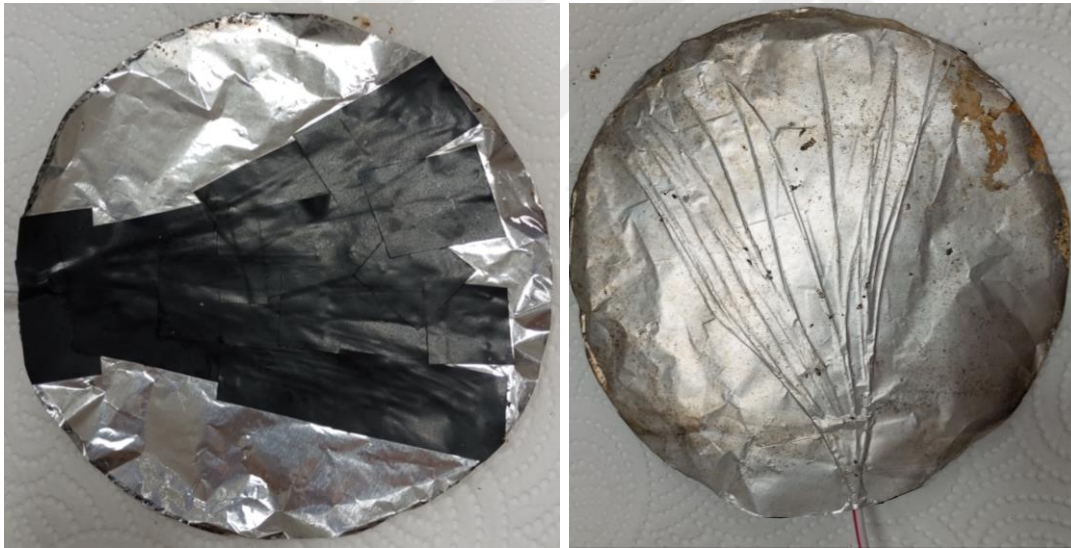
Figure 2.3: Top (left) and bottom (right) view of copper cable glued aluminum foil paper
