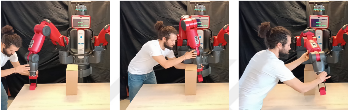
Figure 4.10. Demonstrations of the obstacle avoidance skill are being performed by an expert. Kinesthetic teaching is used to generate sensorimotor demonstrations.
