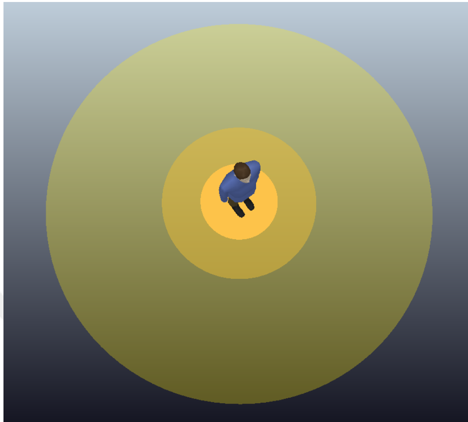
Figure 3.8. Illustration of the proxemics zones. The theory of proxemics defines four notional zones surrounding a human. These zones affect the behavior of the individual by influencing the type and the content of the interaction. These zones (from inner to outer) are Intimate (0-0.5 m.), Personal (0.5-1 m.), Social (1-4 m.), and Public (4-8 m).
