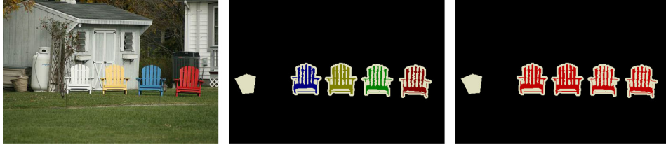
Figure 4.3: Example segmentation from the PASCAL VOC 2012 dataset. The left figure shows the original image from the PASCAL VOC 2012 segmentation dataset. The middle figure depicts the object-level segmentation where the chairs are segmented into distinct regions with colours such as blue, red, green, and yellow, while the background is marked in black. The right panel shows the class-level segmentation, where all chairs are uniformly labelled in red, and the background is depicted in black. [Figure taken from: [7]]
