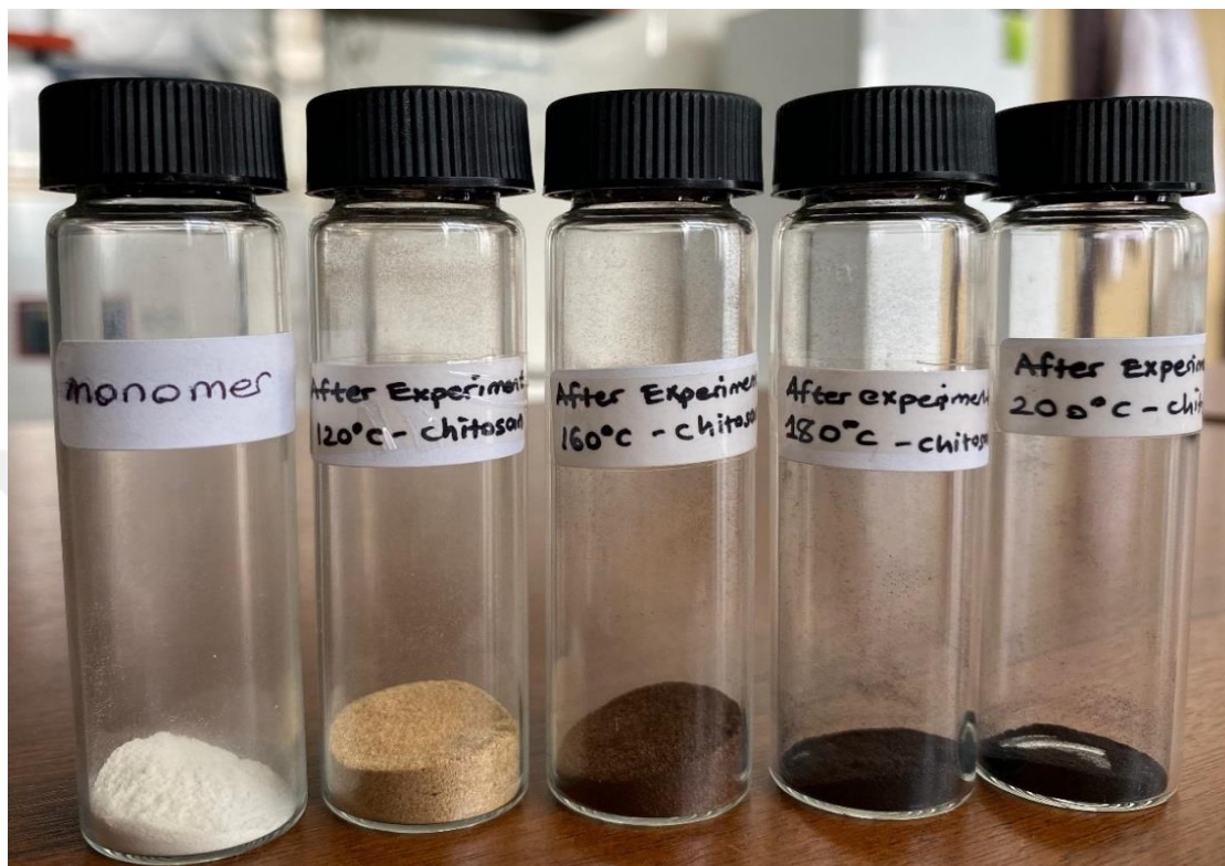
Figure 4.1 Colour changes of the chitosan remaining in the tube from experiments conducted at different temperatures
