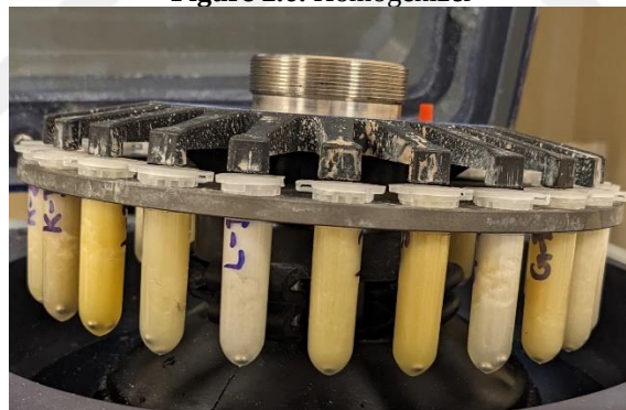
Figure 2.7. Samples in Tubes During the Homogenization Process for Biomarker Analysis
