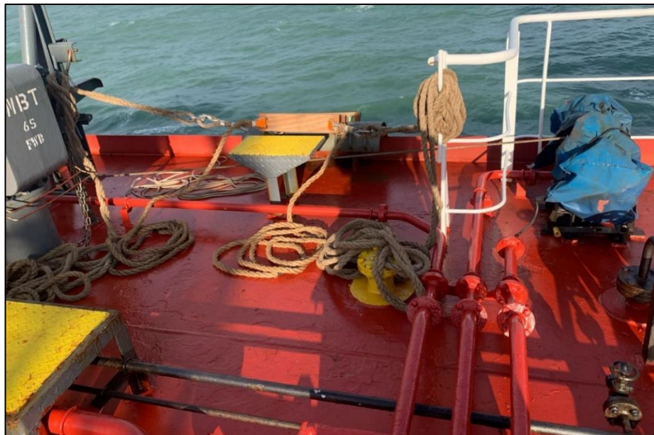
Figure 3.10 : Not secured on deck (Palmers A., 2022)
