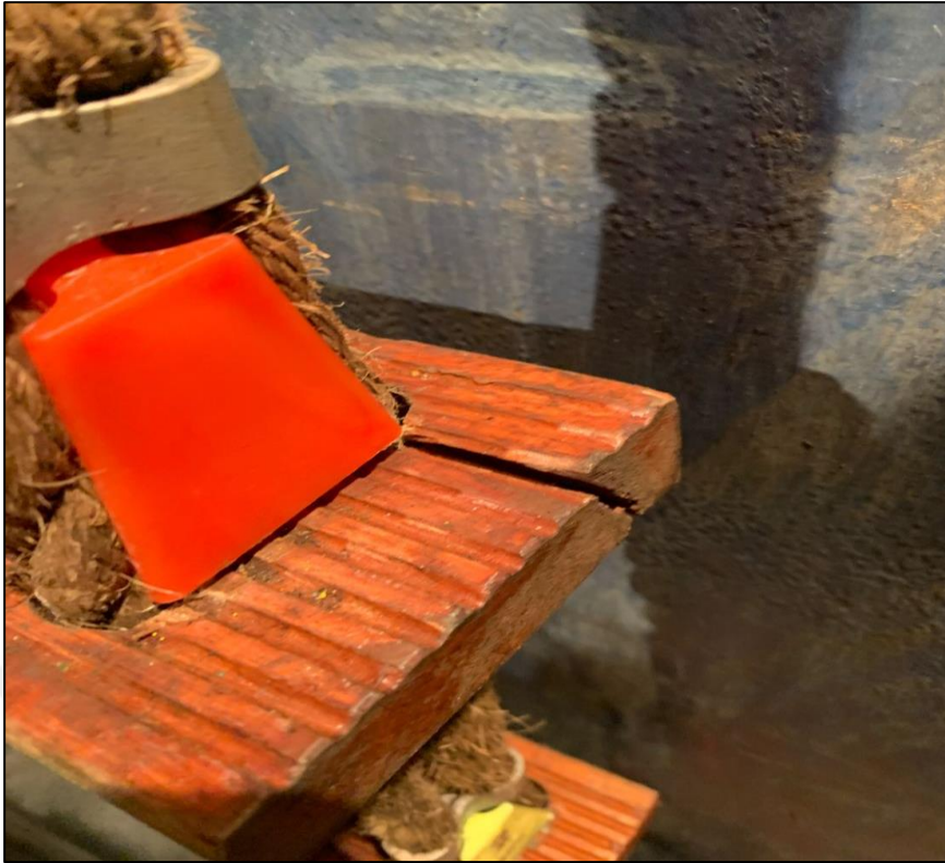
Figure 3.8 : Cracked step (Palmers A., 2022)
