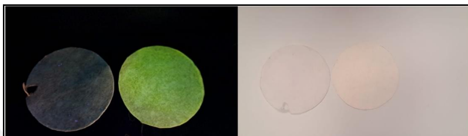
Figure 4.23. Filter papers impregnated 1b photographs in UV (left) and daylight (right) in the absence (left ones) and presence (right ones) of CO.
