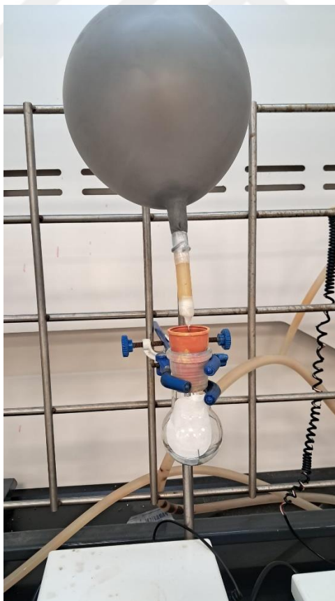
Figure 3.1. Application of CO gas to filter paper in an isolated system.
