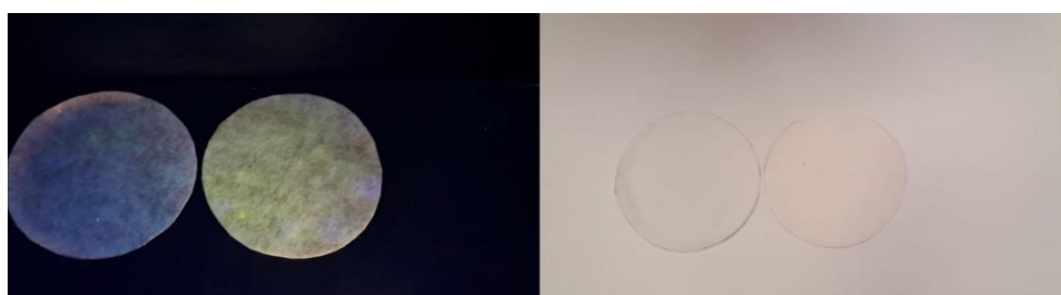
Figure 4.63. Filter papers impregnated 1e photographs in UV (left) and daylight (right) in the absence (left ones) and presence (right ones) of CO.
