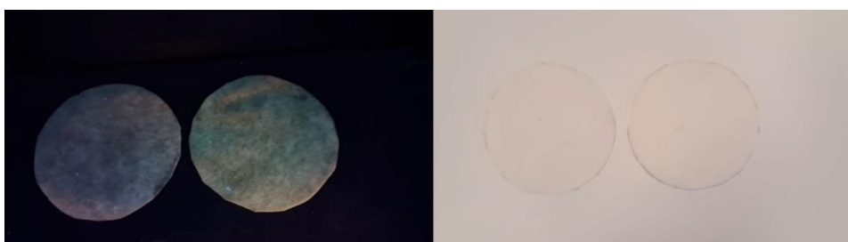
Figure 4.37. Filter papers impregnated 1c photographs in UV (left) and daylight (right) in the absence (left ones) and presence (right ones) of CO.
