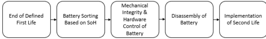
Figure 3.5: Second Life Cycle of Batteries without Permanent Interconnection
