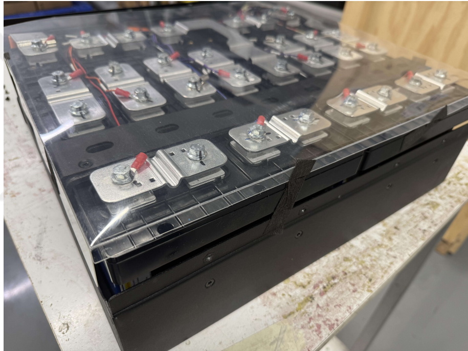
Figure 3.4: Bolted Prismatic Batteries without Permanent Interconnection
