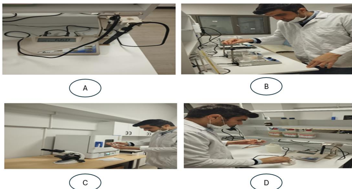
Figure 3. 8. A. pH meter apparatus, B. homogenization of the meat sample with distal water, C. the meat sample after being homogenized, D. measuring the pH value of the sample
