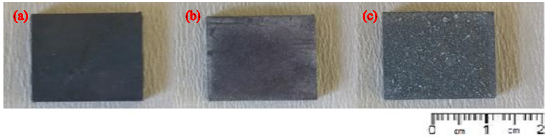
Figure 14: Plates coated 1mM Sr added solution: (a) Plate at 9 th day of immersion, (b) Plate at 14 th day of immersion; (c) Plate at 18 th day of immersion.
