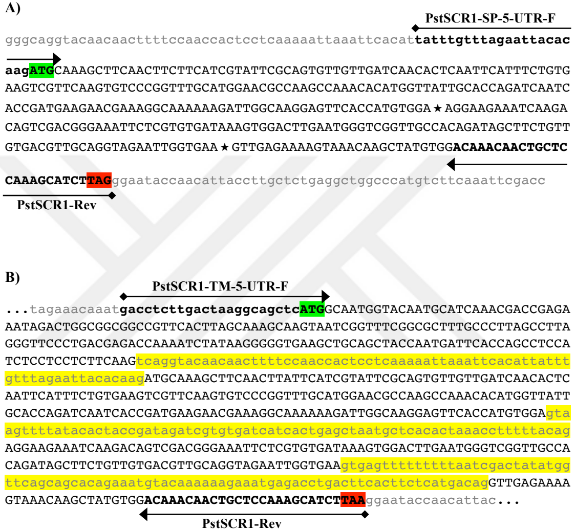
Figure 3.4 PCR primer design strategy to detect the presence of PstSCR1 expression in Pst infected wheat samples. A) PstSCR1 EST sequence; arrows indicate primers annealing regions and expected amplification size is 375 bp. Stars indicate the exon joints. B) The genome region of predicted transcript sequence of PstSCR1 homolog and introns are highlighted in yellow. Expected spliced product amplification size is 560 bp when all introns are removed (Table 2.3).
