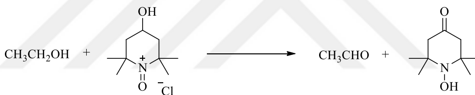
Scheme 13. First study of oxoammonium salts used in oxidation of alcohols
