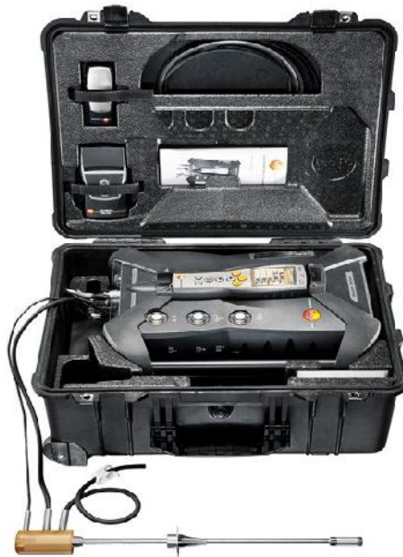
Figure 3.43. Picture of testo 350 gas analyser.
