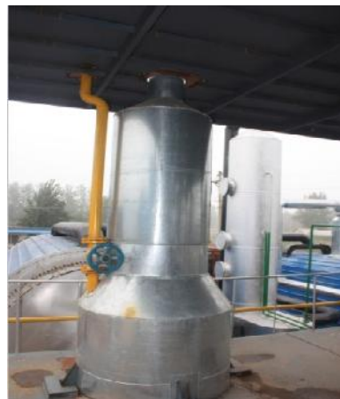
Figure 3.16. Gas separator system.
