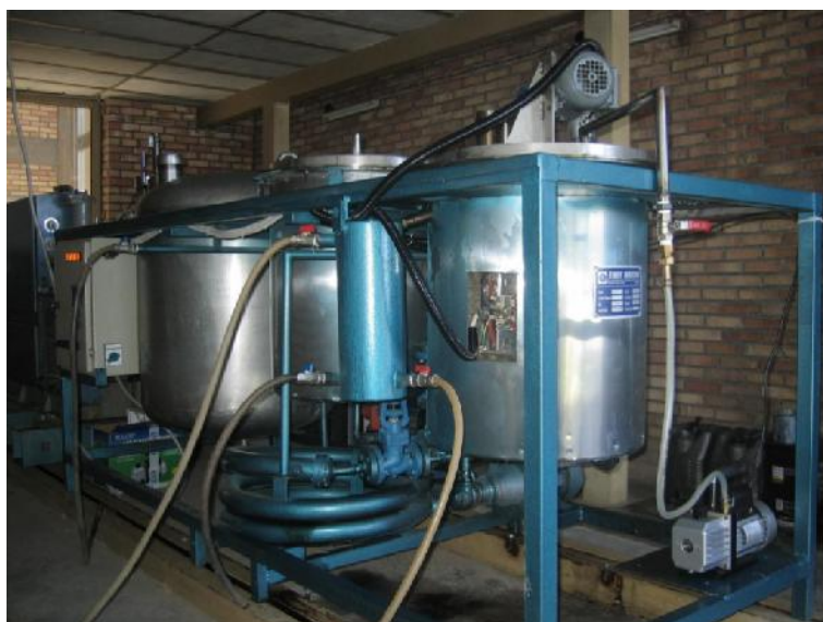
Figure 3.2. Picture of the batch reactor pyrolysis system.
