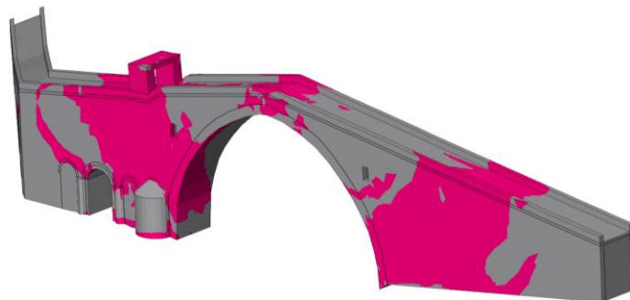
Figure 5.65 : Principle tensile stresses after last converged load-step (pink: \geq 0.3\text{MPa} , Grey: < 0.3\text{MPa} ), downstream.
