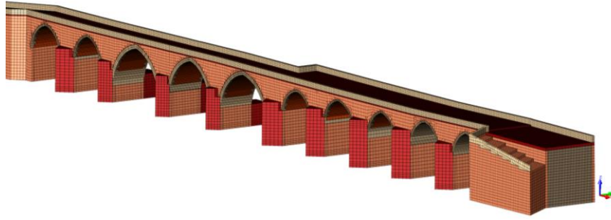
Figure 4.6 : 3D modeling of Dicle (On Gozlu) Bridge with fine mesh-upstream.
