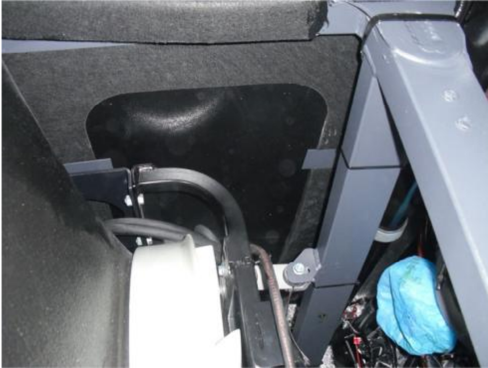
Figure 4.9. Insulation in the engine compartment for large surfaces to the passenger compartment, but not for chassis beams
