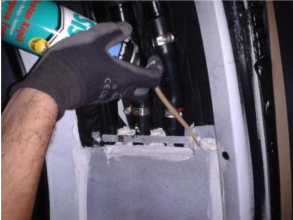
Figure 4.11. Filling of the corners of travel busses with PU foam
