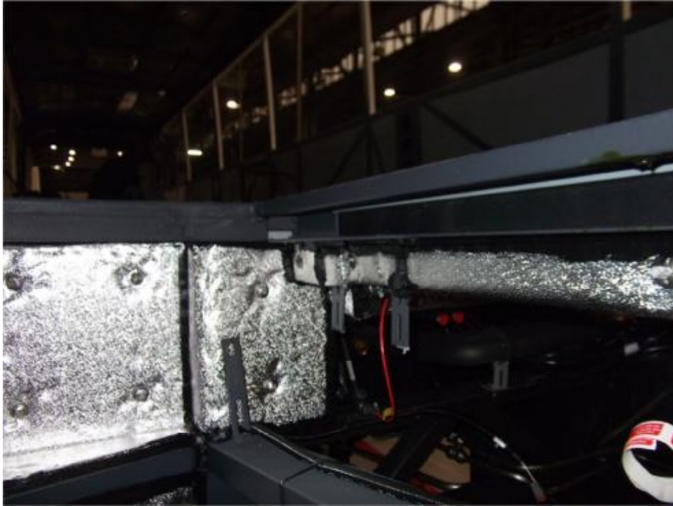
Figure 4.10. Heat reflecting surface in the engine compartment
