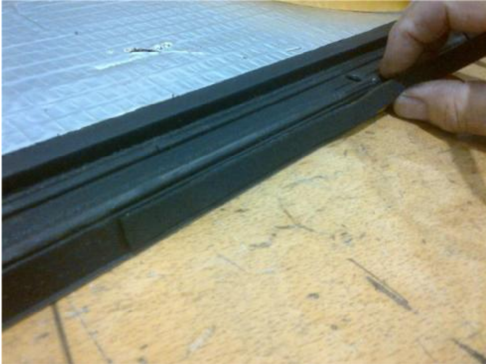
Figure 4.4. Sealing tape 9010 all around the conical outline of the four floor panels in the rear
