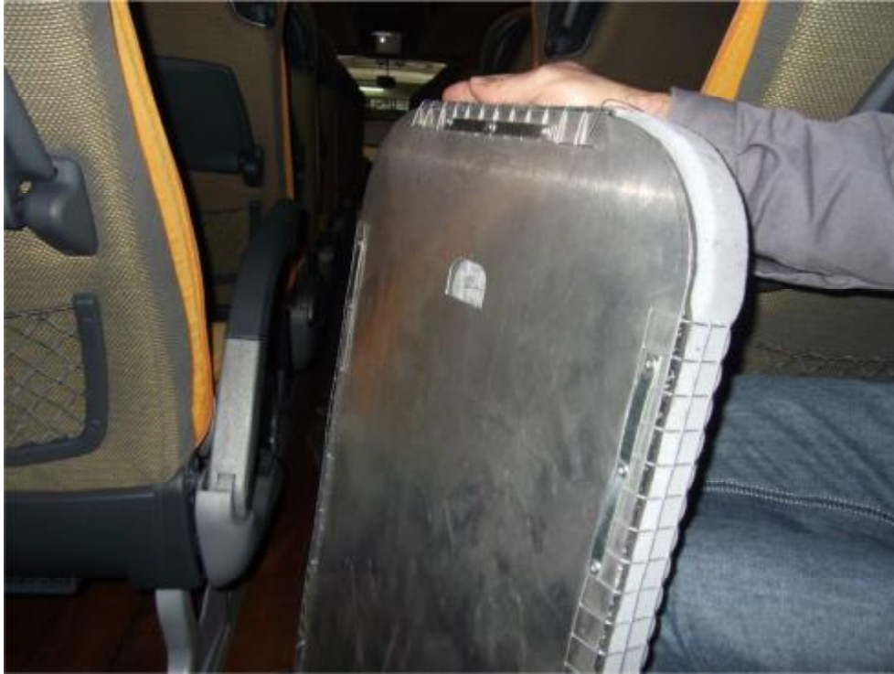
Figure 4.3. Lid in the floor with reflecting surface to the engine compartment and insulation
