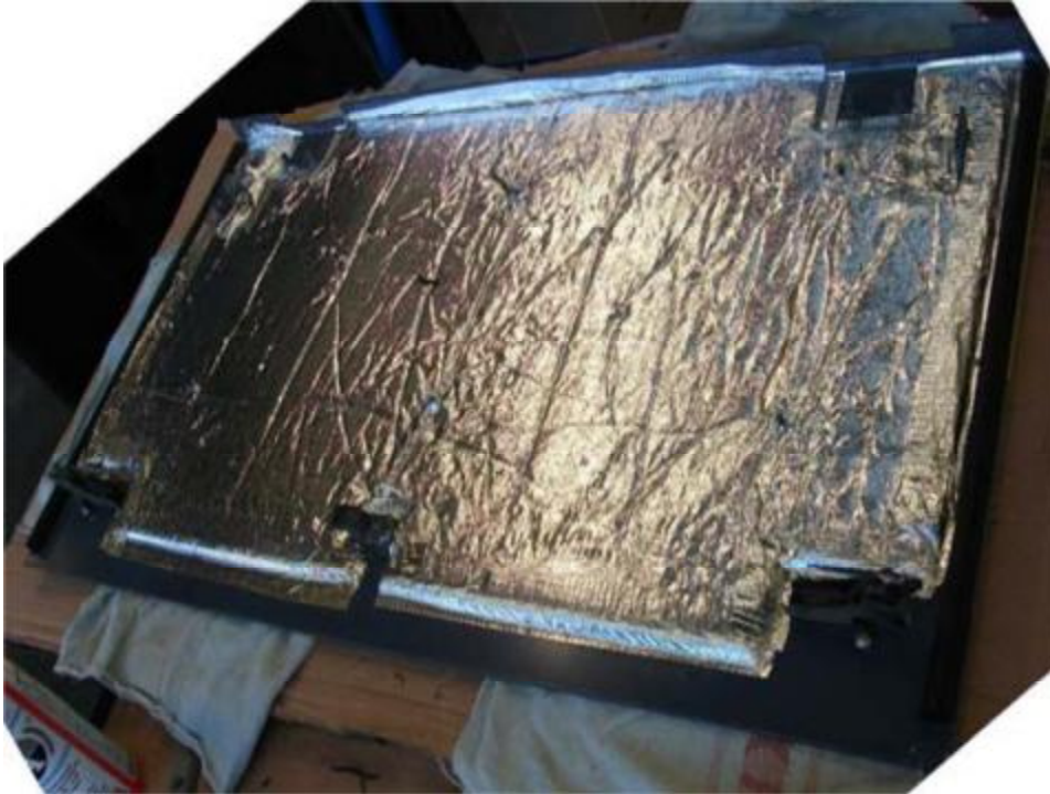
Figure 4.7. Maintenance flap with heat reflecting surface and insulation to the engine compartment
