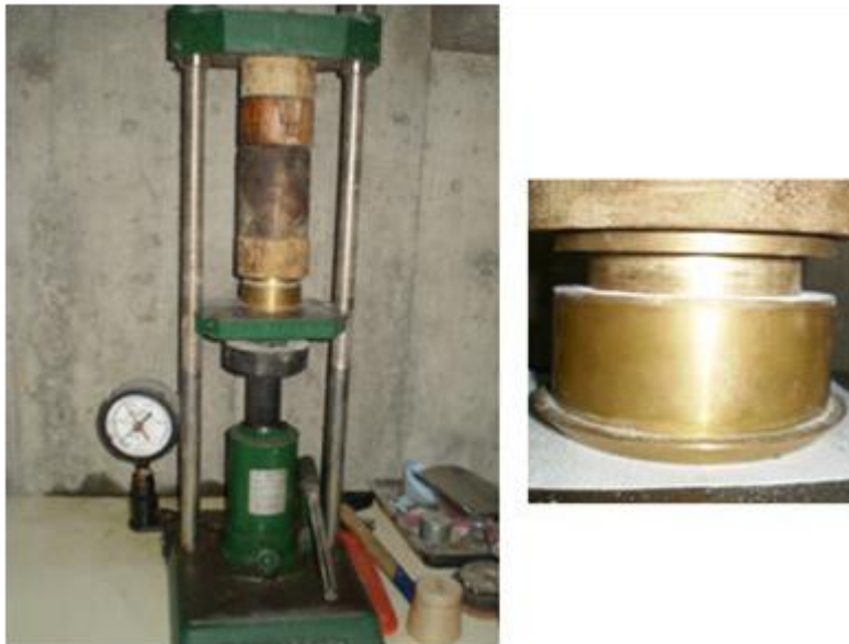
Figure 3.28 A View of Static Compaction with the Hydraulic Jack
