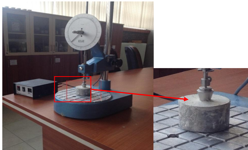
Figure 3.6.b A view of fall cone test
