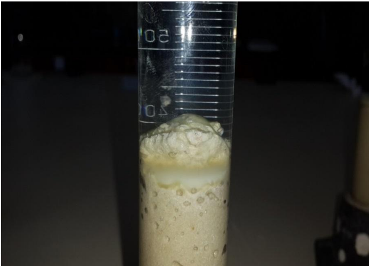
Figure 3.23 Formation of mud which prevent water penetration into lower layers
