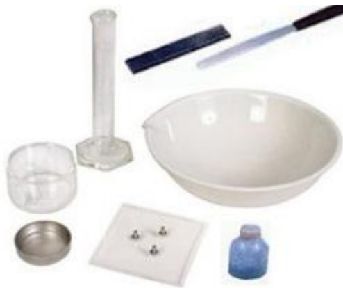
Figure 3.9 Set up used to determine SL
