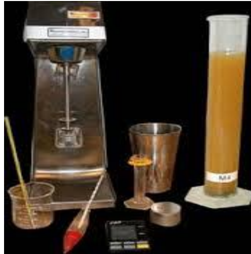
Figure 3.2a Determination of grain size distribution via Hydrometer test
