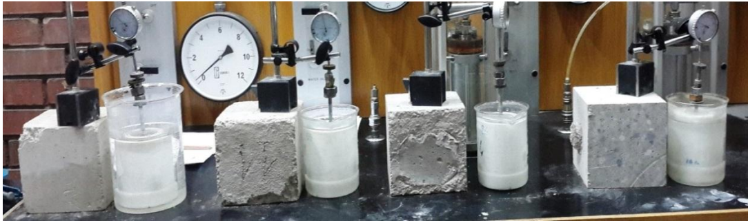
Figure 3.21 A view of free swelling test
