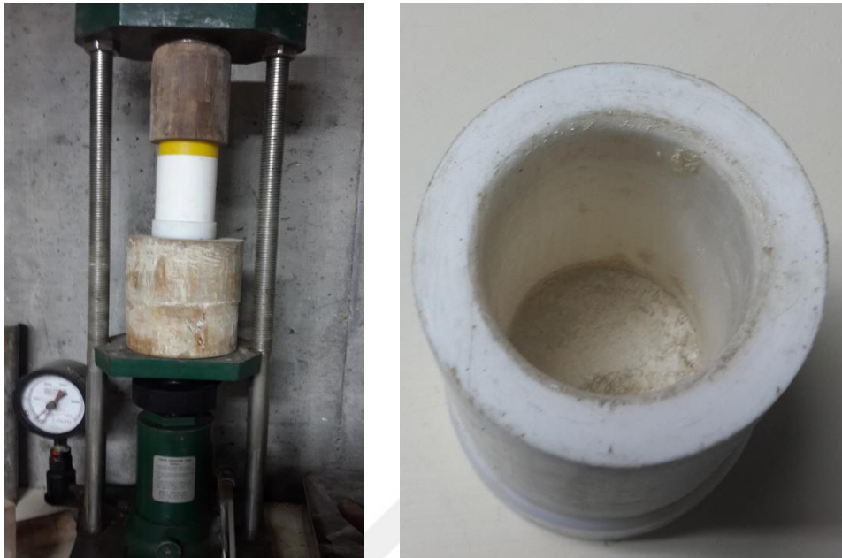
Figure 3.19 Hydraulic jack used to compact samples for free swell test and prepared test sample
