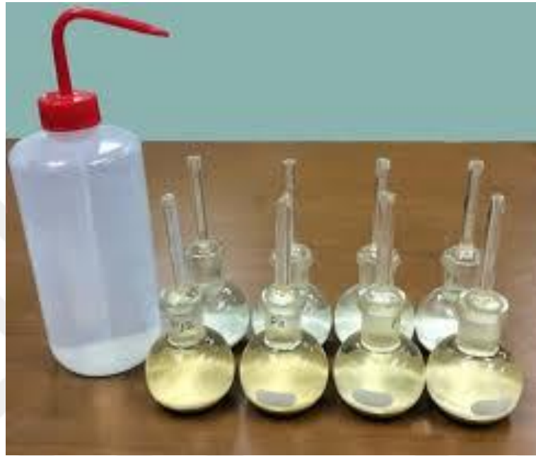
Figure 3.10 A view from soil specific gravity test
