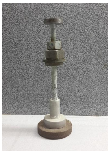
Figure 3.17 A view of axial load applying device with attached porous stone and extra weights
