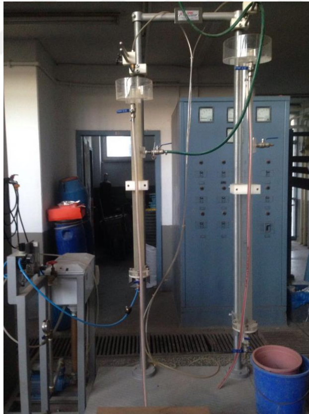
Figure 4.6 Experimental setup of column flotation
