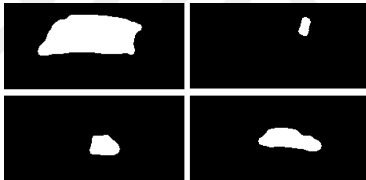
Figure 2.2. Examples of the silhouettes based on ABL background subtraction along with morphological operations. The images were cropped from the omnidirectional images for better visualization. The silhouettes at top-left: van, top-right: pedestrian, down-left: motorcycle, down-right: car.
