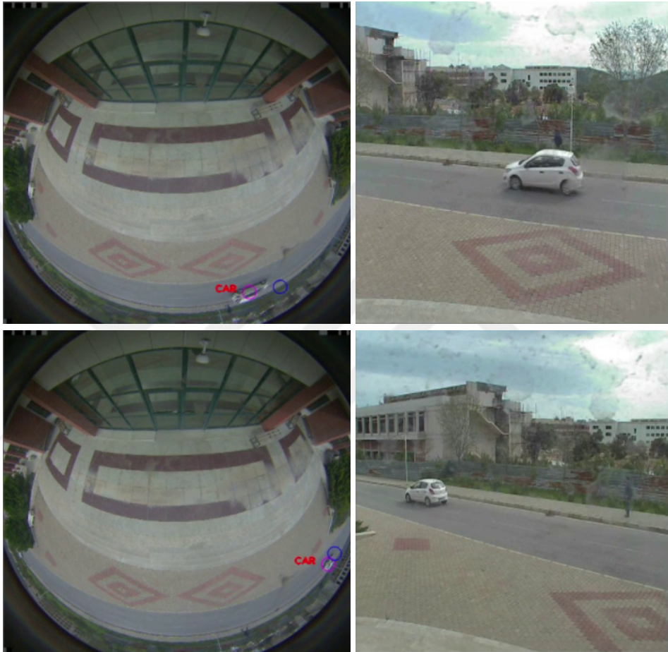
Figure 5.5. Example of car tracking. Purple circles indicate the location after updated with the formula given in Equation 4.3.
