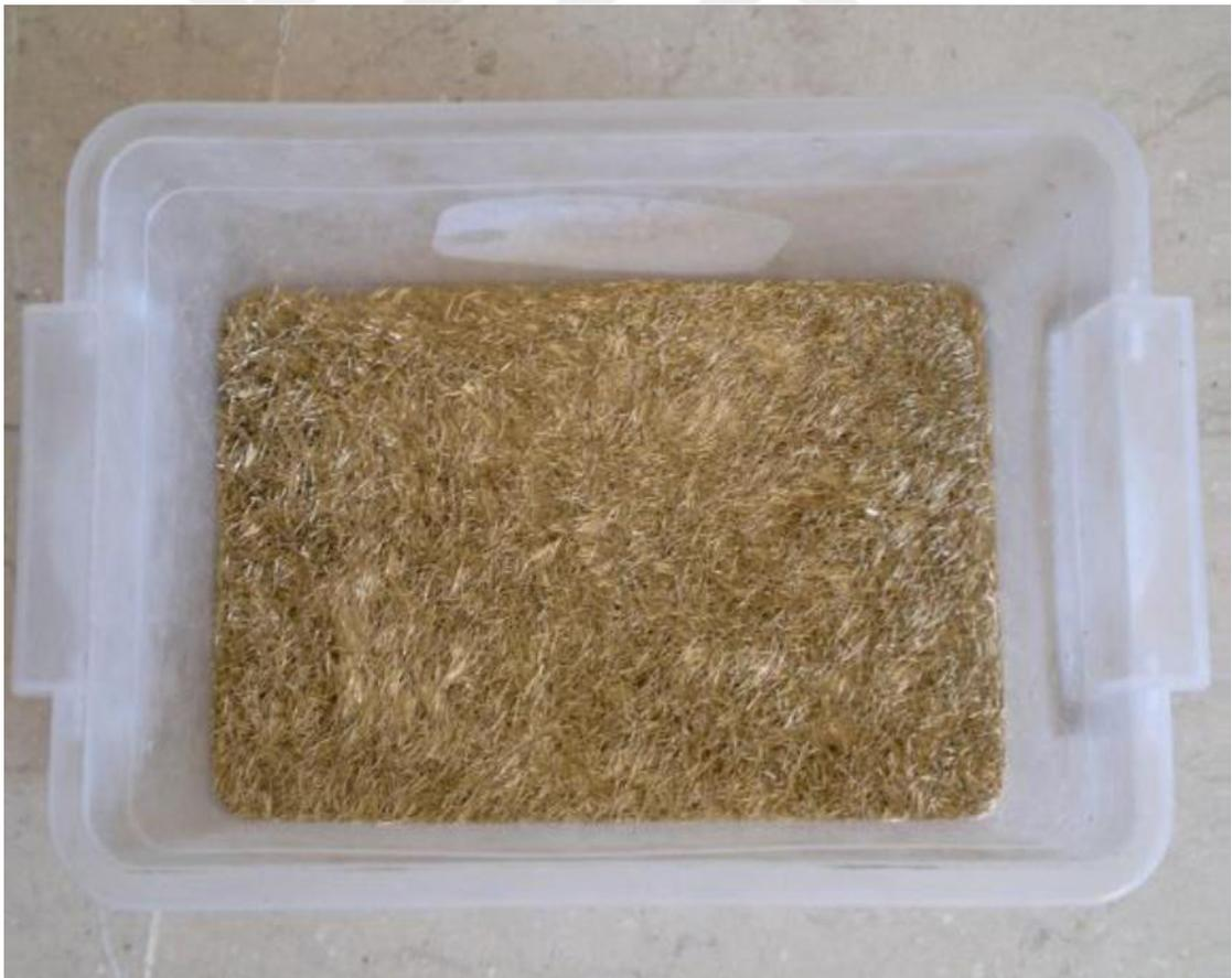
Figure 3.1 Micro steel fibers.
