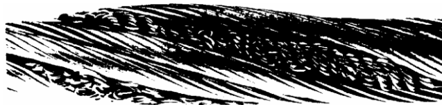
Figure 4.9 : Local increase in diameter of rope (Southwest Wire Rope Inc., 2008).
