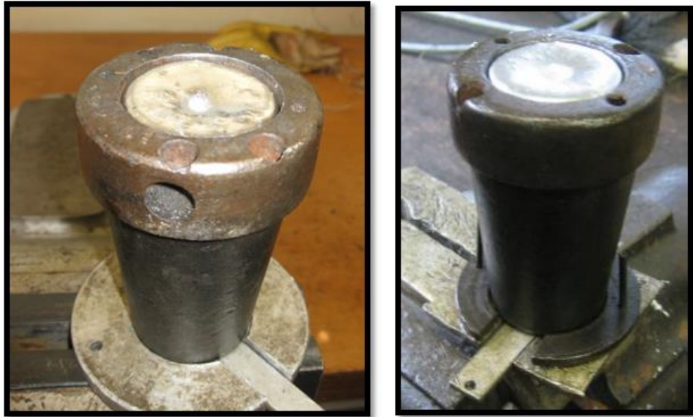
Figure 5.12 : Wire rope end when cast process finish.
