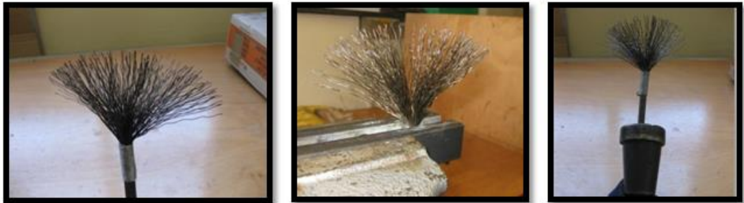
Figure 5.6 : Separated region of wire rope.
