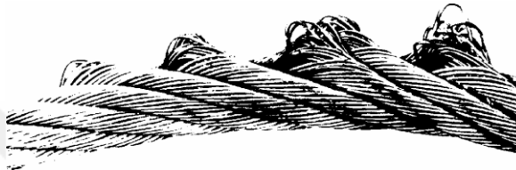
Figure 4.8 : Examples of wire extrusion (Southwest Wire Rope Inc., 2008).
