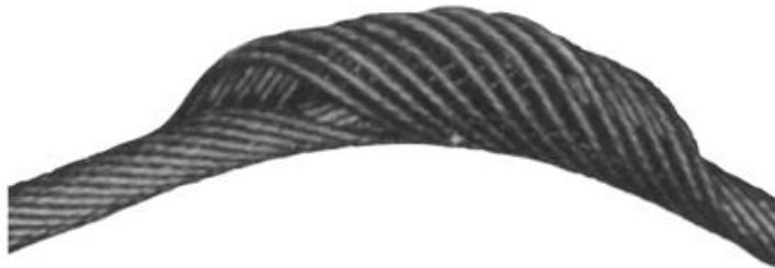
Figure 4.6 : Birdcage (Southwest Wire Rope Inc., 2008).
