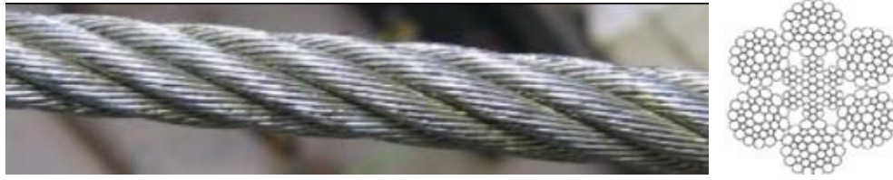
Figure 5.1 : 6 x 36 Warrington Seale wire rope sample and its cross section view.
