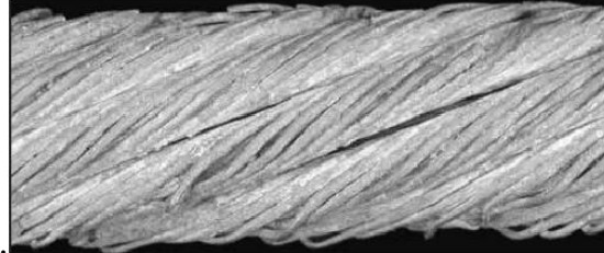
Figure 4.18 : Wire rope exposed to high temperature (Verreet & Ridge, 2005).
