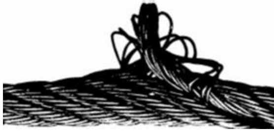
Figure 4.7 : Strand extrusion (Southwest Wire Rope Inc., 2008).
