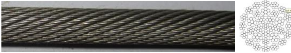
Figure 5.2 : 32(W) x 7 soliflex strands rotation resistant wire rope sample.
