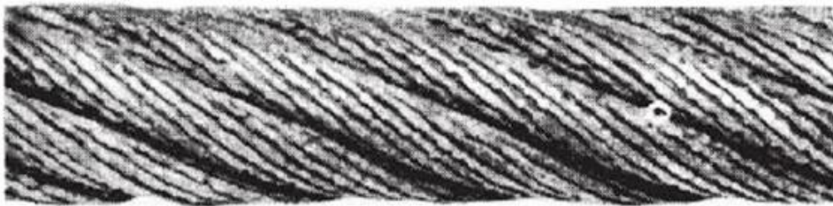
Figure 4.3 : Corroded rope (Southwest Wire Rope Inc., 2008).
