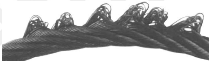
Figure 4.14 : Loop formations (Southwest Wire Rope Inc., 2008).
