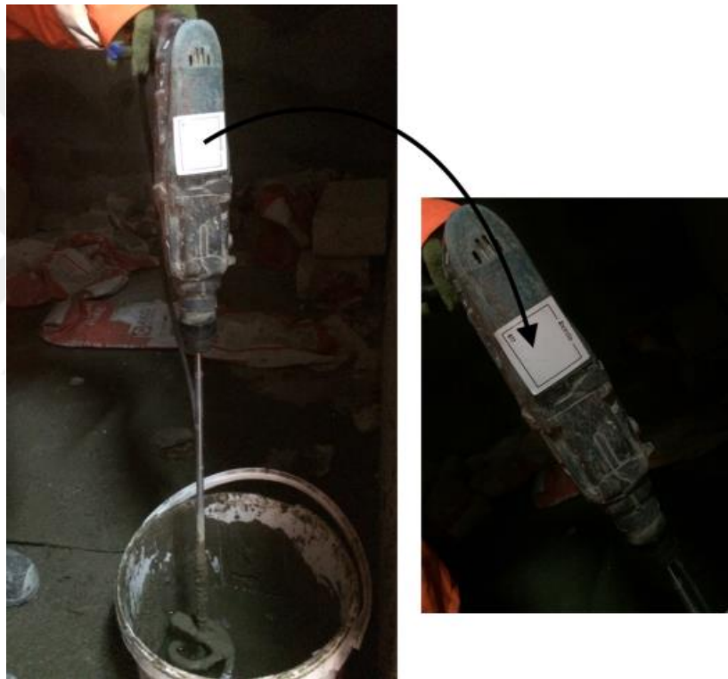
Figure 4.9 : RFID tag on the hand drill.
