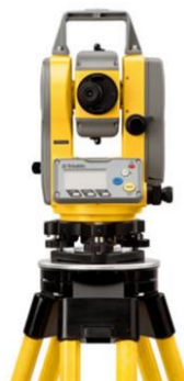
Figure 2.15 : A total station used for building construction layout and alignment (Url-9).
