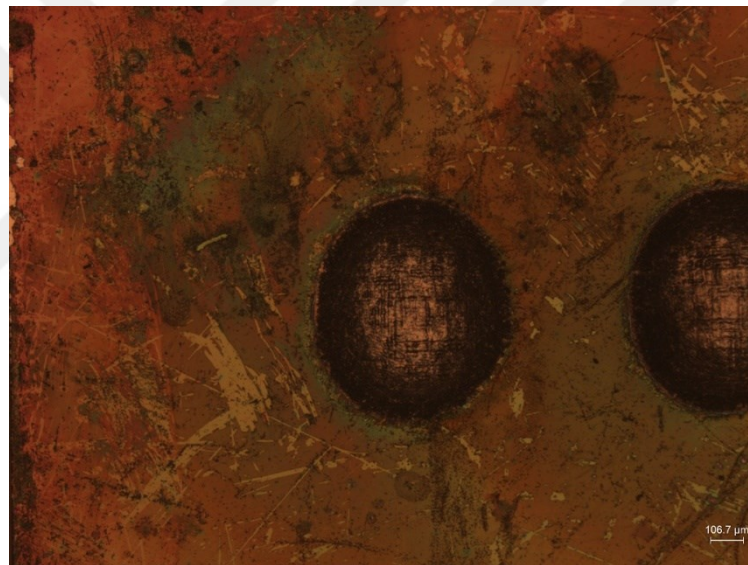
Figure 3.13 Microscope image of the crater after 30 consecutive laser shots
