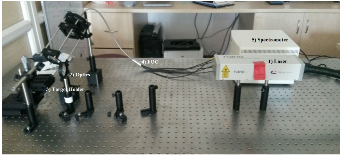
Figure 2.7 The LIBS apparatus used in this study
