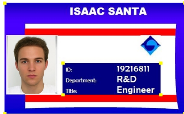
Figure 2.4. Location of eight synchronization points in identity document for image rectification. (Yellow squares)
