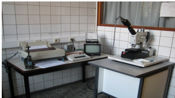
Figure 4.7: Conventional micro hardness test device.
