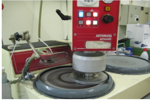
Figure 4.5: Automatic grinding and polishing machine.
