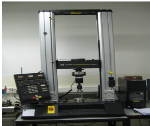
Figure 4.6: A picture of the Instron compression machine.
