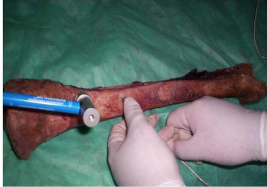
Figure 1. Measurement of FRFs on fresh-frozen tibial bone
