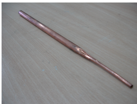
Figure 4.21 One of the open ends sealed empty copper tube with an outer diameter of 6.40 mm (for the MgB 2 /Fe/Cu 6 filament wire production).
