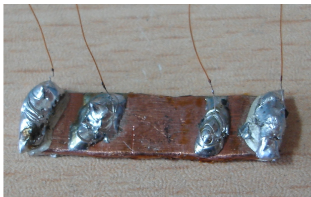
Figure 5.73 Current and voltage contacts of MgB 2 /Fe/Cu multifilament tape.
