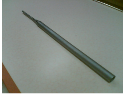
Figure 4.13 One of the open ends sealed empty iron tube with an outer diameter of 10.6 mm (for the MgB 2 /Ag/Fe 7 filament wire production).
