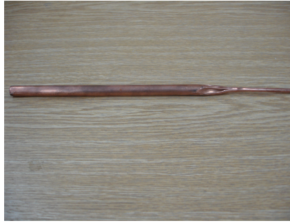
Figure 4.19 One of the open ends sealed empty copper tube with an outer diameter of 10 mm (for the \text{MgB}_2/\text{Fe}/\text{Cu} 6 filament wire production).
