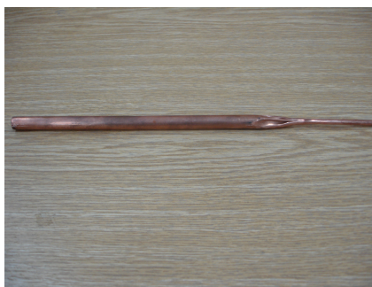
Figure 4.22 One of the open ends sealed empty copper tube with an outer diameter of 10 mm (for the \text{MgB}_2/\text{Fe}/\text{Cu} 7 filament wire production).
