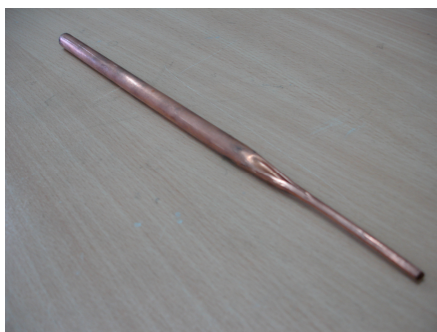
Figure 4.24 One of the open ends sealed empty copper tube with an outer diameter of 6.40 mm (for the \text{MgB}_2/\text{Fe}/\text{Cu} 7 filament wire production).
