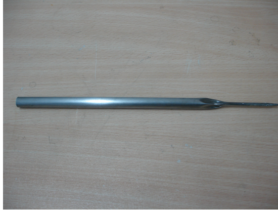
Figure 4.15 One of the open ends sealed empty iron tube with an outer diameter of 10.6 mm (for the \text{MgB}_2/\text{Fe} monofilament wire production).
