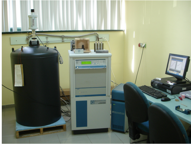
Figure 4.33 Quantum Design Physical Property Measurement System (PPMS) and Vibrating Sample Magnetometer (VSM) System.
