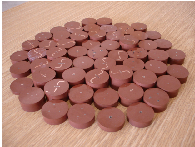
Figure 4.30 MgB 2 wires and tapes which were compressed with copper bakelite powder.
