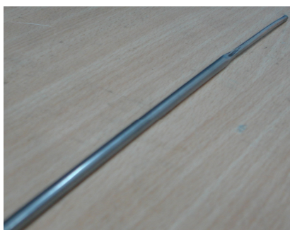
Figure 4.17 One of the open ends sealed empty iron tube with an outer diameter of 4.95 mm (for the MgB 2 /Fe monofilament wire production).
