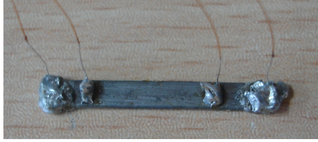
Figure 5.3 Current and voltage contacts of MgB 2 /Fe monofilament tape.
