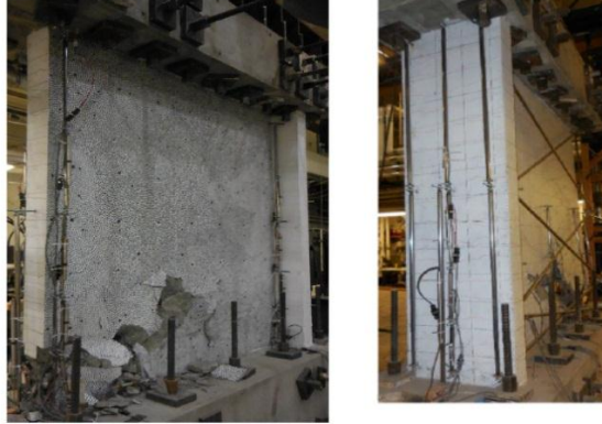
Figure 3.18 : Segura (2017) – WP4 east and west boundary final damage state.
