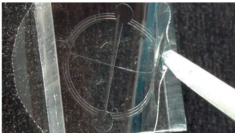
SI Figure 3.2: Photograph of the transverse plane microfluidics formed in a thin PDMS layer. The layer is transferred to a thicker one for punching process, which defines the trap chamber.
