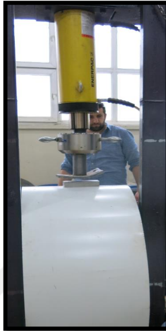
Figure 3.4. Dent implementation of the models
