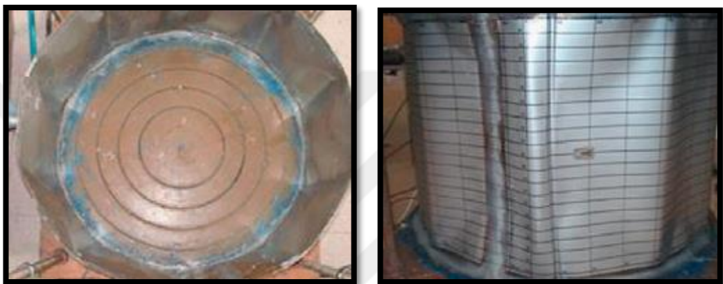
Figure 2.5. Collapse modes of research by Fatemi et al. (2013)
