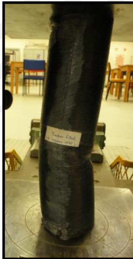
Figure 2.13. Failure mode in research by Tohid Ghanbari Ghazijahani et al. (2015d)
