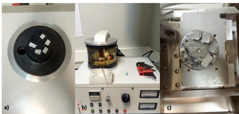
Figure 5.2. The coating process of the samples before SEM: a) Uncoated nanofiber samples, b) Polaron SC7640 Sputter Coater, c) Coated samples on the SEM tab.
