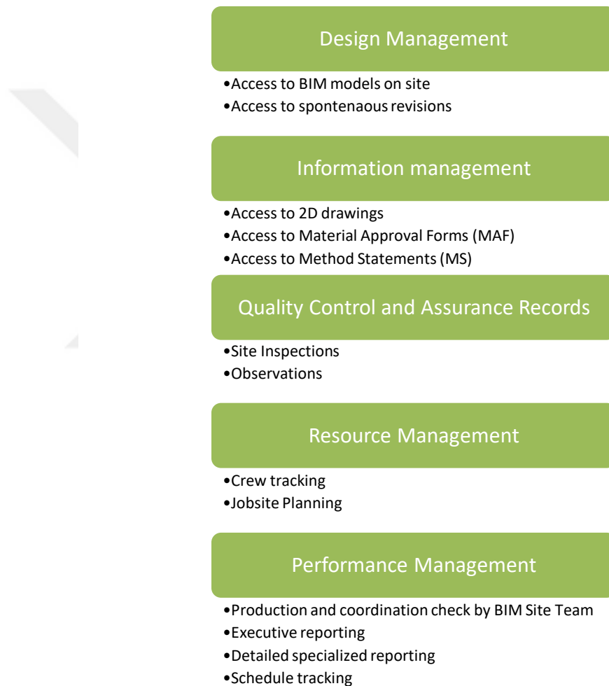
Figure 3.12 : Use cases enabled by mobile BIM implementation.
