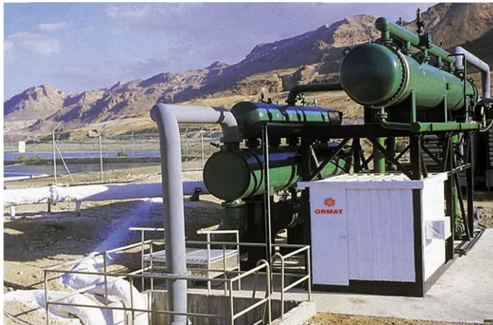
Figure 1.2: The 150 kW solar pond and power unit at the Dead Sea, Israel [5].
