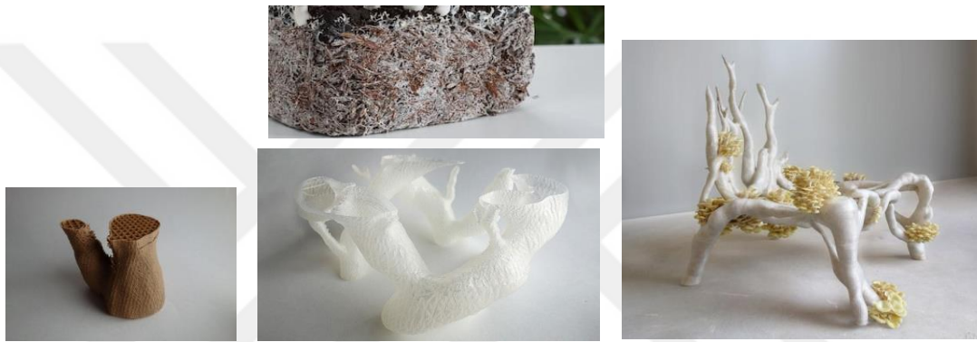
Fig 5.38: 3D printed mycelium infused straw, 3D printed outershell and mushrooms growing from the mycelium and straw filled shell (URL - 33)
