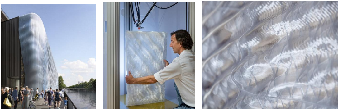
Fig 5.21: Polycarbonate Facade testing (URL – 19)
