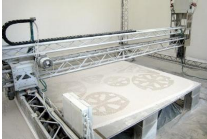
Fig 4.3: D Shape binder jetting process (URL – 36)
