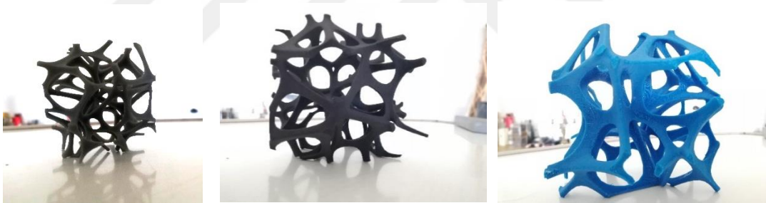
Fig 5.40: a. Structure printed with SLA tech. b. Structure printed with MJF tech. c. Structure printed with FDM tech. (Provided by the author)
