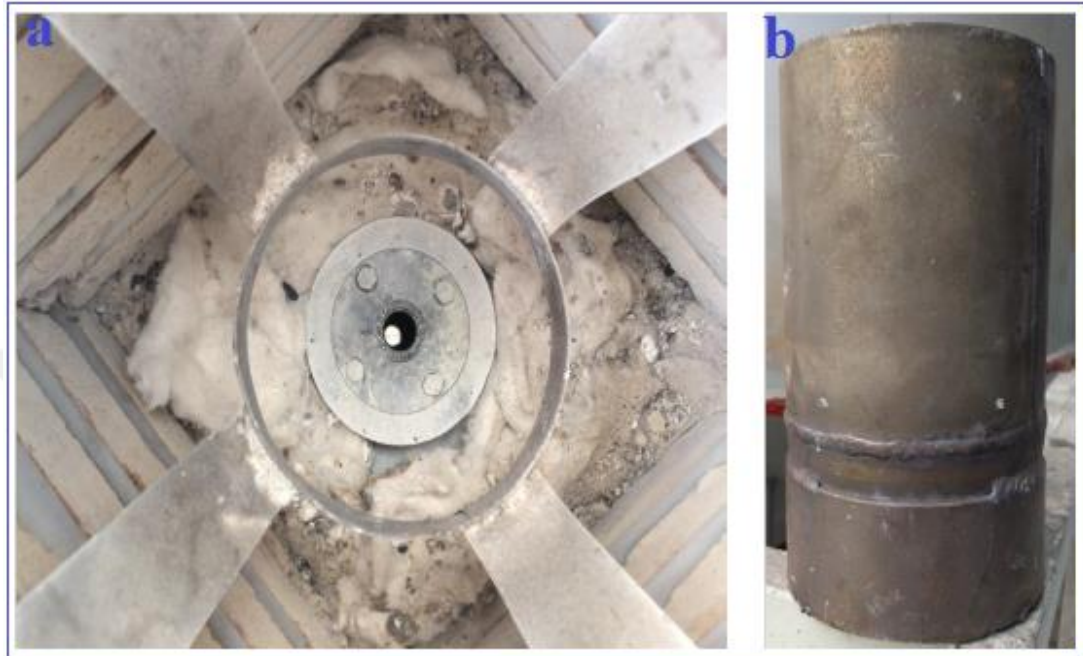
Figure 8.2. (a) Image of the interior of the melting furnace, (b) Melting pot.
