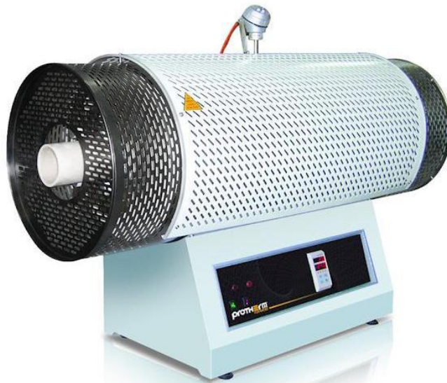
Figure 8.17. Atmosphere controlled heat treatment furnace (PTF 16/80/610).
