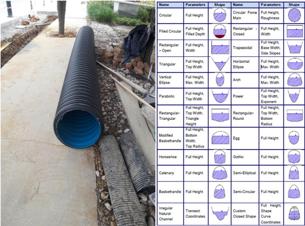
Figure 4.3: Sample cross sections in SWMM and sample pipe type of the ITU drainage system.
