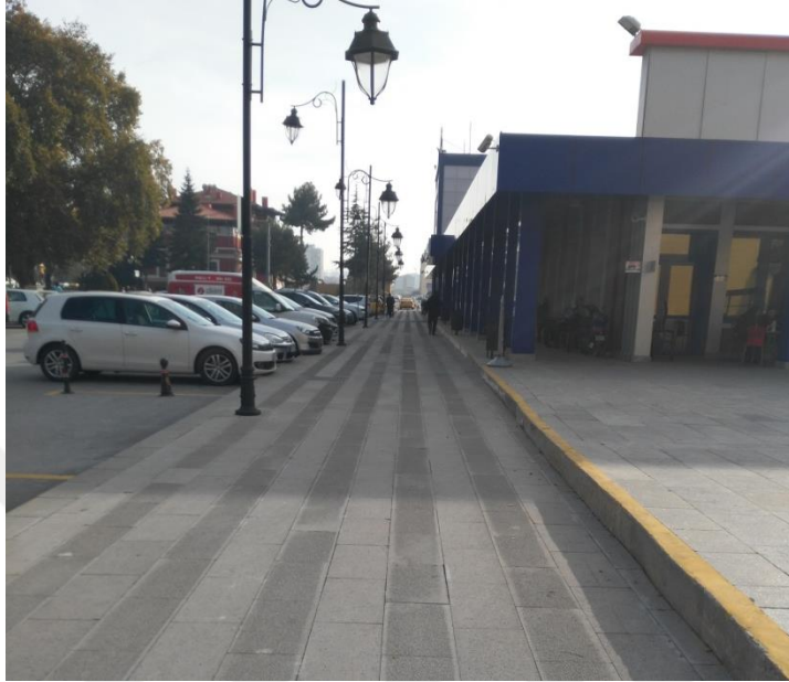
Figure 4.9. Well designed pavements in terms of width, height and level changes
