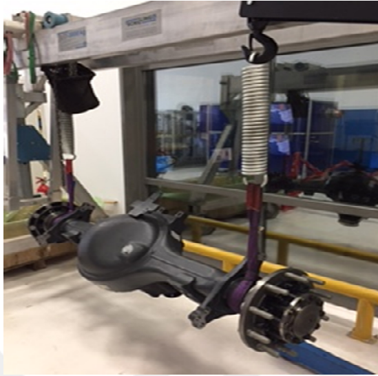
Figure 3. 28: Rear axle suspended with soft springs.
