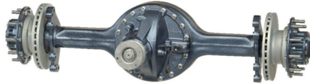
Figure 3. 4: Banjo type rear axle [32].
