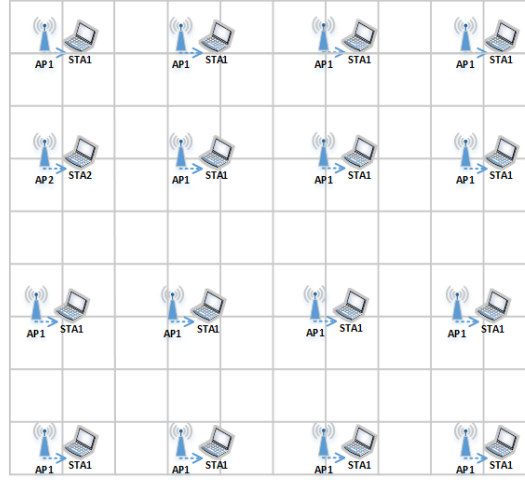
Figure 3.9 : 16 AP-STA pair grid network deployment
