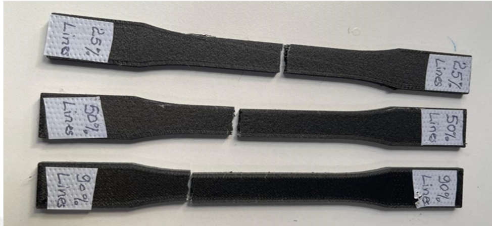
Figure 4.3: The sample of the infill pattern is Lines with different infill densities: a) 25%, b) 50%, and c) 90% after the breaking point
