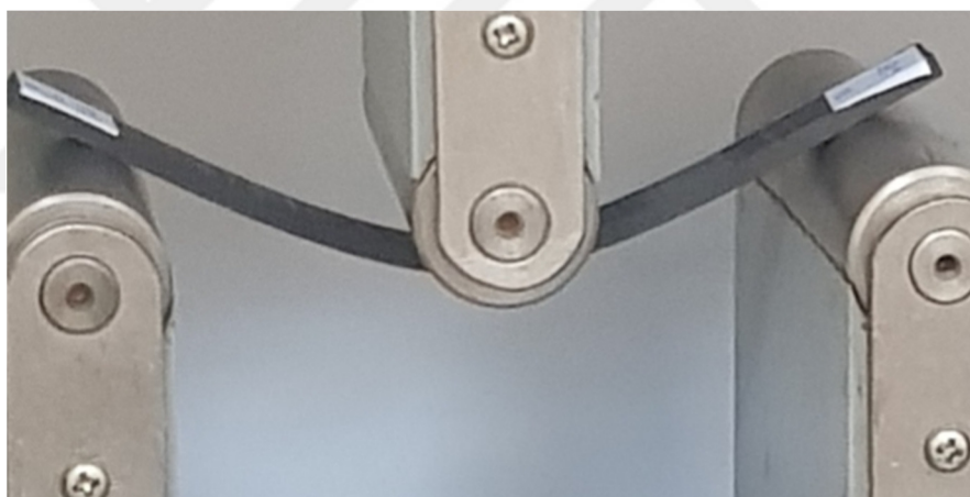
Figure 4.16: The three-point bending test of PA12-CF as a sample according to the ASTM D790
