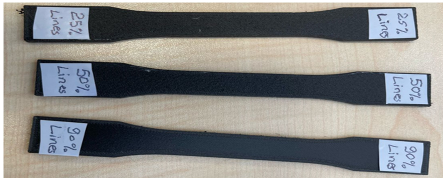
Figure 4.1: Fabricated tensile test samples
