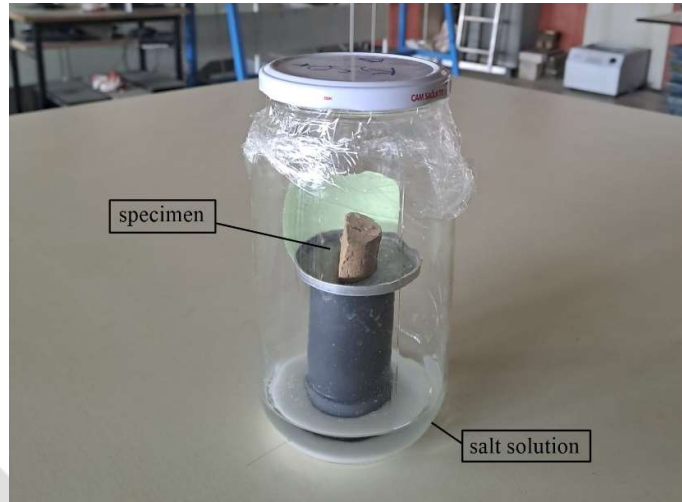
Figure 4.10. Vapor equilibrium specimens on stands inside jars
