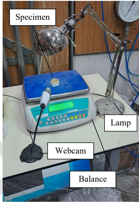
Figure 4.1. Evaporation test setup
