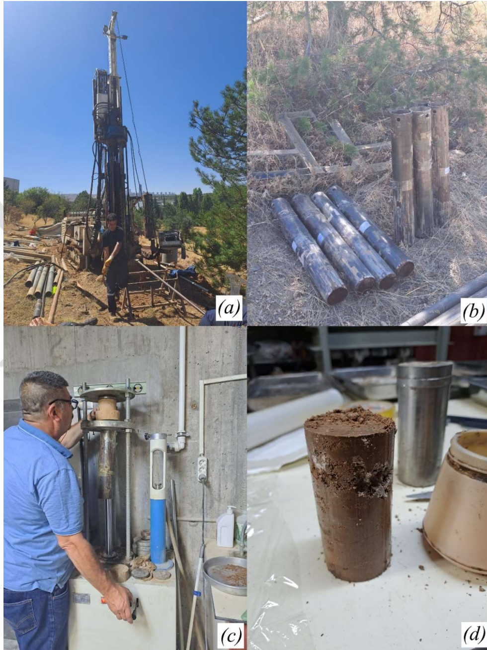
Figure A.1. (a) Sample extraction at the METU site, (b) samples in shelby tubes at the METU site, (c) specimen extrusion in the lab and (d) problematic specimen extruded from the Bahçelievler sample
