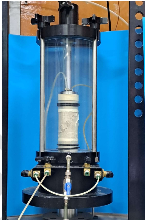
Figure 5.11. Unsaturated UU triaxial setup with air drainage valve open
