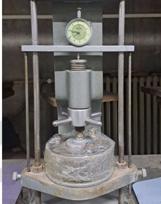
Figure 5.9. Oedometer test setup for unsaturated specimens
