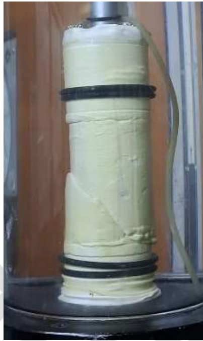
Figure 5.4. Failure plane in CD triaxial test on METU specimen
