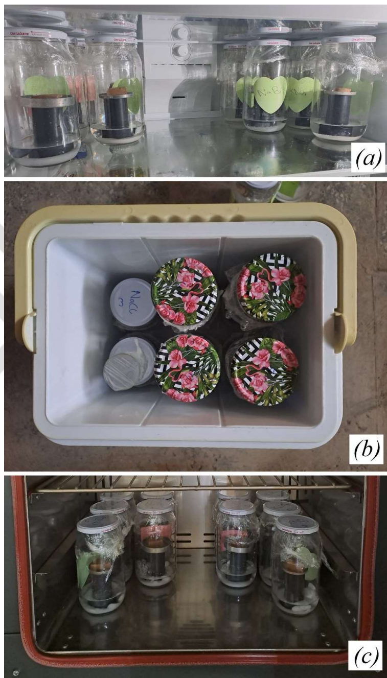
Figure A.3. Temperature chambers for vapor equilibrium: (a) refrigerator, (b) ice-box, (c) low temperature oven
