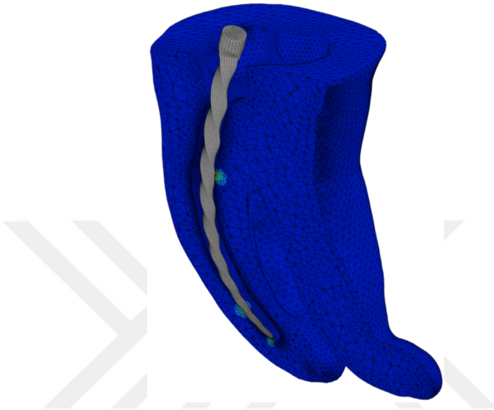
Figure 7.18. Dentin von Mises stress distribution at the end of insertion step.
