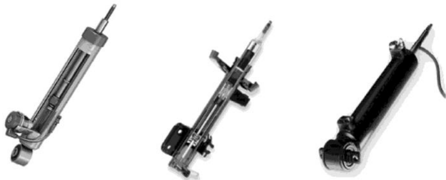
Figure 4 From left to right: solenoid valve EH damper from Sachs, MR damper from Delphi and ER damper from Fludicon.
