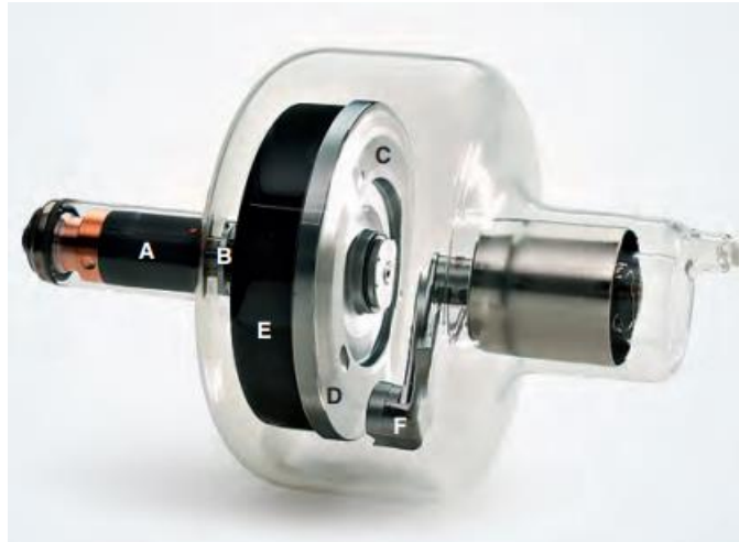
Figure 3.2. X-ray target displaying rotor (A), stem (B), and molybdenum-alloy target (C) with tungsten-rhenium alloy track (D) for X-ray production. The graphite heat sink (E) and the cathode cup (F), which houses the tungsten filament © Plansee SE (X-ray tube manufactured by Dunlee), are also depicted
