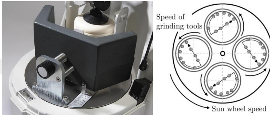
Figure 5.5. Planetary ball mill (a) and (b) schematic of cataract movement during milling
