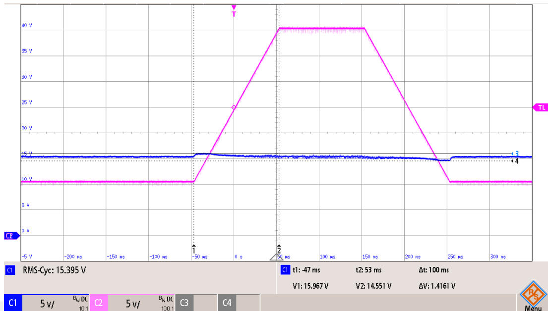
Figure 3.8 Effect of input voltage variation
